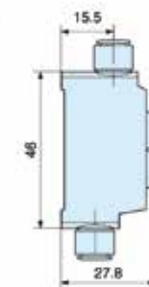
swivel elbow push-in connector 4 mm OD tube
